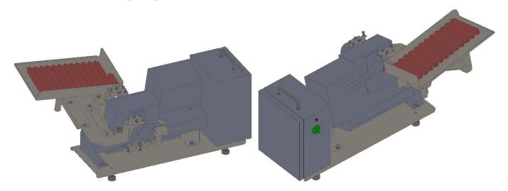
OVERVIEW: This device is utilized in food factories and similar settings to swiftly and effectively create perforations in packaging film for paste products, facilitating easy removal of the film.
