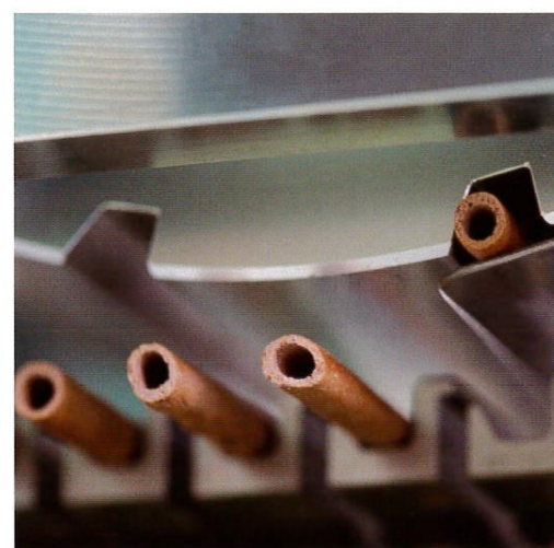
Accurately grasps the product and carries it to the nozzle side
