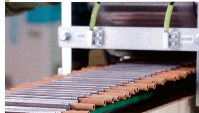
Line up and feed one by one to ensure accurate filling.
