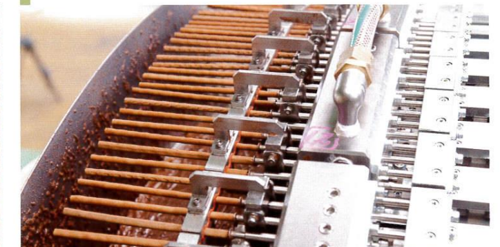
Filling is completed in about 3 seconds from one side.
