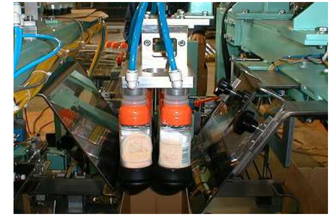
Bottle is transferred and packaged using a 2 axis robot
