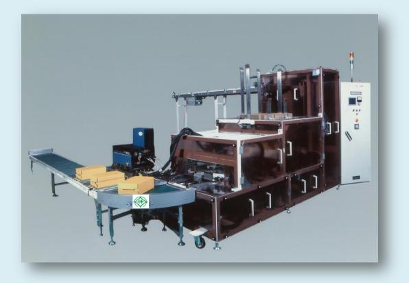
Until now, goods which have been packed by carton box sometimes have cracks and thus incurred loss in the manufacturing chain. This machine has been used to pack products by cardboard without making damage. It has led to reduce the box material cost. Moreover, the shock has been optimized to protect the damage of the products during transportation.
