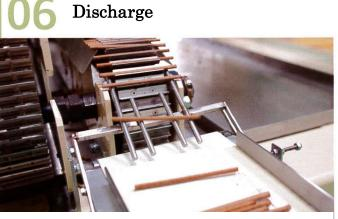
Products come from the delivery conveyor is sent to the dispatch conveyor
