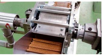
If there is any gap in feeding through conveyor, then it refills the blank in every 0.05 seconds.
